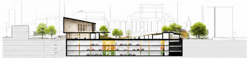
LONGITUDINAL SECTION – UNDERGROUND PARKING 1/300
